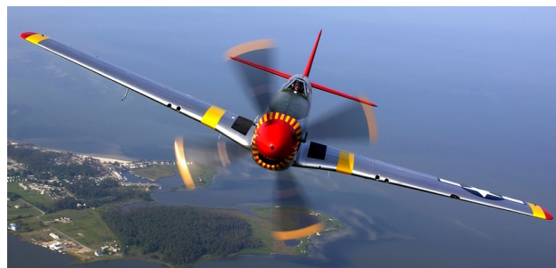
Figure 1: Example of a four bladed propeller driven aircraft - North American P51 Mustang
